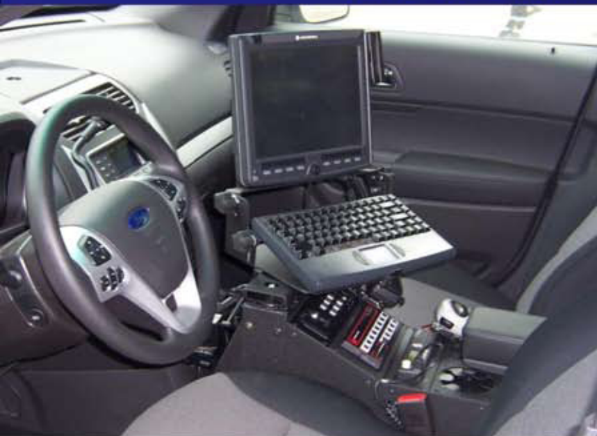
CC-MC-18 console with CM-UMNT-SA-M810 in new Ford U.V.
