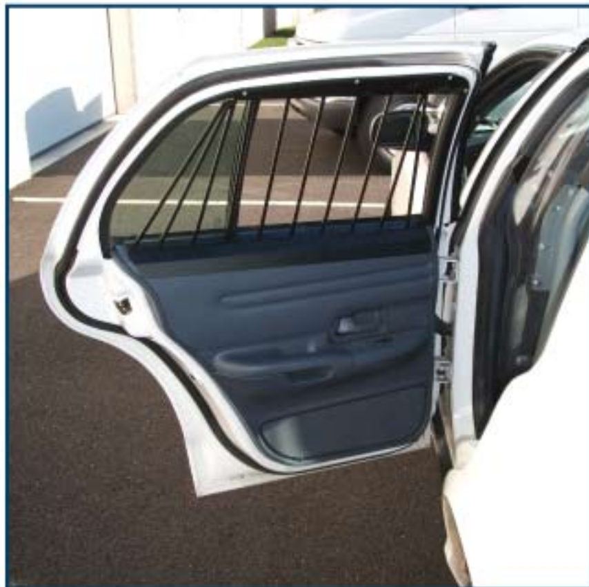
Interior Window Bars allow for excellent driver visibility and easy cleaning.
