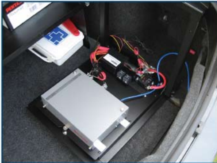
Safely mount important equipment: Havis fold-down trunk side mounts allows important electronic devices to be safely mounted in a secure area. (C-TSM-CHGR-P shown)
