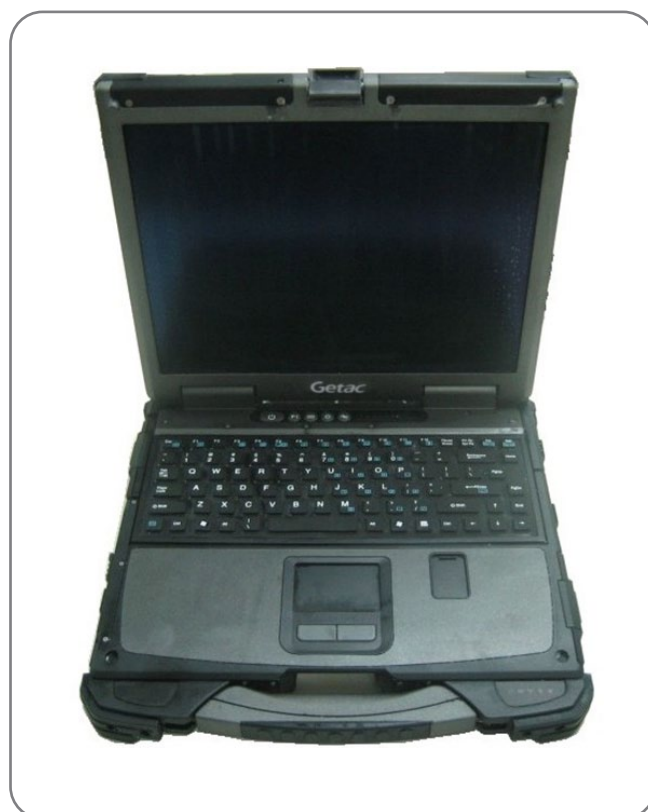
[Figure 5] Post-Salt Fog Test B300 After Water Wash
